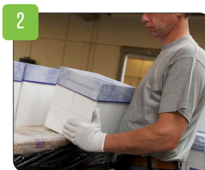
2 Pull and push the box around the lower layer to avoid lifting.
