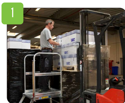
1 Use technical aids to get a proper working height.
