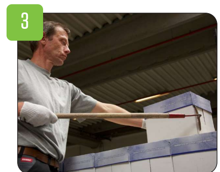
3 Use a reach tool to pull the boxes far back closer to you.
