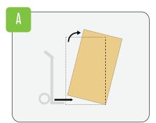
Tip the box slightly forward and push the platform of the sack trolley under it.
