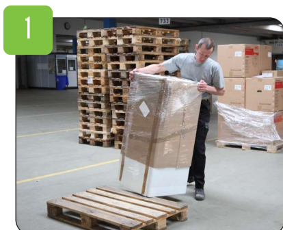
Tip, edge and twist the load upwards until one corner is supported by the pallet.
