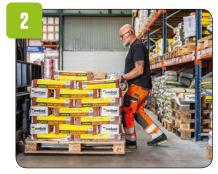
**Tip no. 2:** Pull the pallet clear of the rack to allow you to work in an upright posture with at least 1 x 1 metre free space in the work area.
